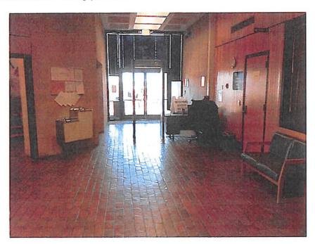
5. None of the exterior doors are equipped with intrusion alarms for notification of a breach of the building after hours. This issue is complicated by the fact that the building is accessed after normal business hours for use by employees of the probation office. A controlled access keycard system would provide both the necessary access and required security for both exterior and interior doors.
